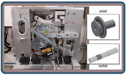
In cooperation with TU Braunschweig, the test rig is used for the experimental investigation of radial air bearings radial air bearings for the analysis of static and dynamic properties in the low speed range. Some specifications of the test rig can be listed as follows:
