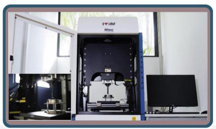
A tribometer is a machine used to perform tests of wear, friction and lubrication that underlies tribology. Conducting tests using tribometers is particularly effective in investigating the friction pairing of coated surfaces in bearings.
