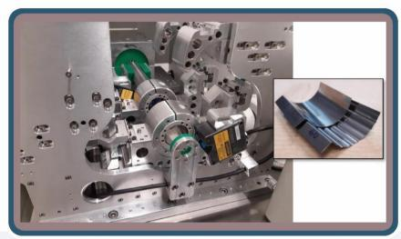
In cooperation with the TU Braunschweig, the test rig is used for the experimental investigation of radial air bearings for the analysis of various static and dynamic properties in the high-speed range. Some specifications of the test rig can be listed as follows:
